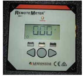
Solar Panel Battery Monitor
